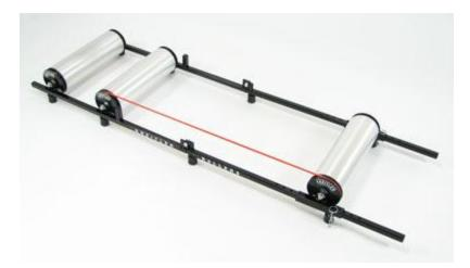
A rubber belt connects the front drum with the front drum from the rear wheel. As you pedal your bike, it turns the rear drums which in turn drive the front drum and turns your front wheel. As you can imagine, it takes some practice to learn
